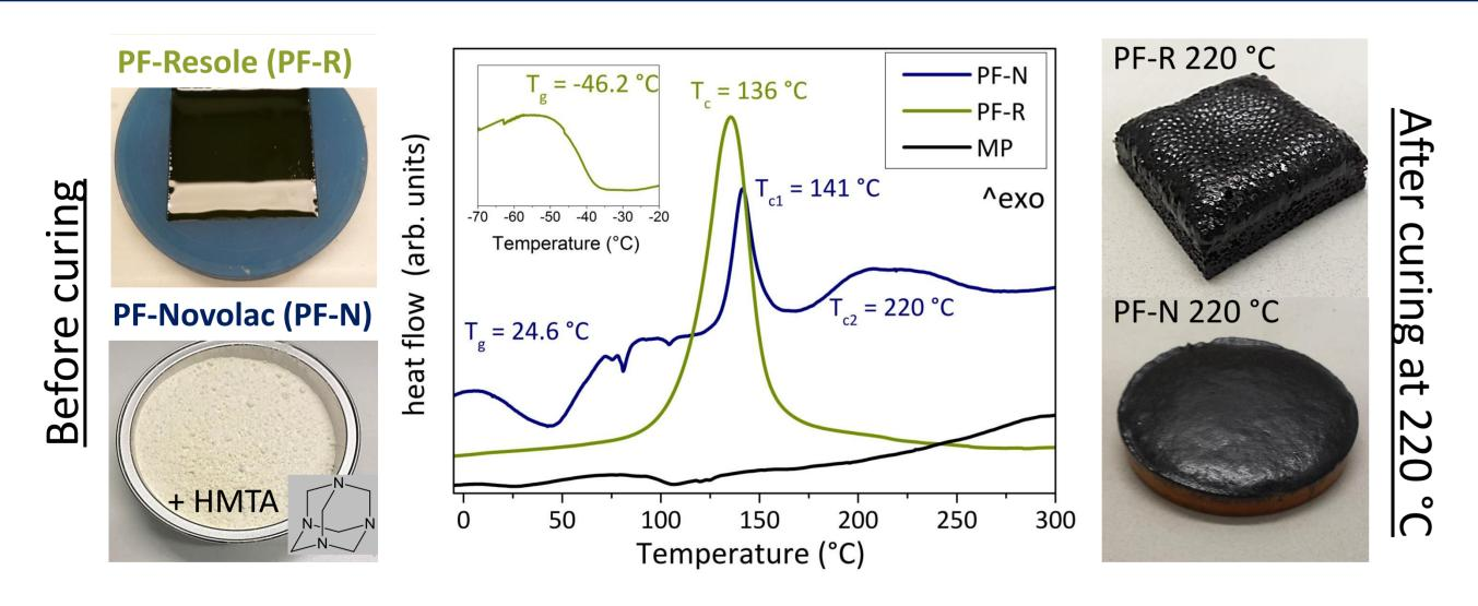
Differential scanning calorimetry (DSC);  $T_g$  glass transition temperature;  $T_c$  reaction temperature; HMTA: hexamethylenetetramine = curing agent
