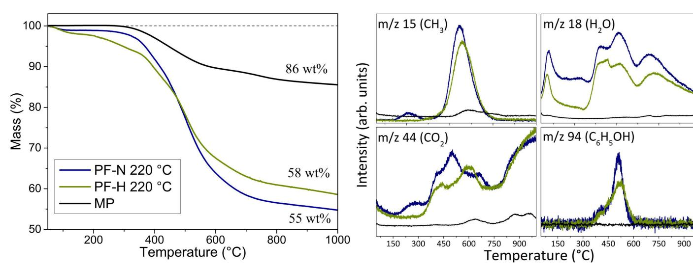
Thermogravimetric Analysis coupled with Mass Spectroscopy (TG-MS)
