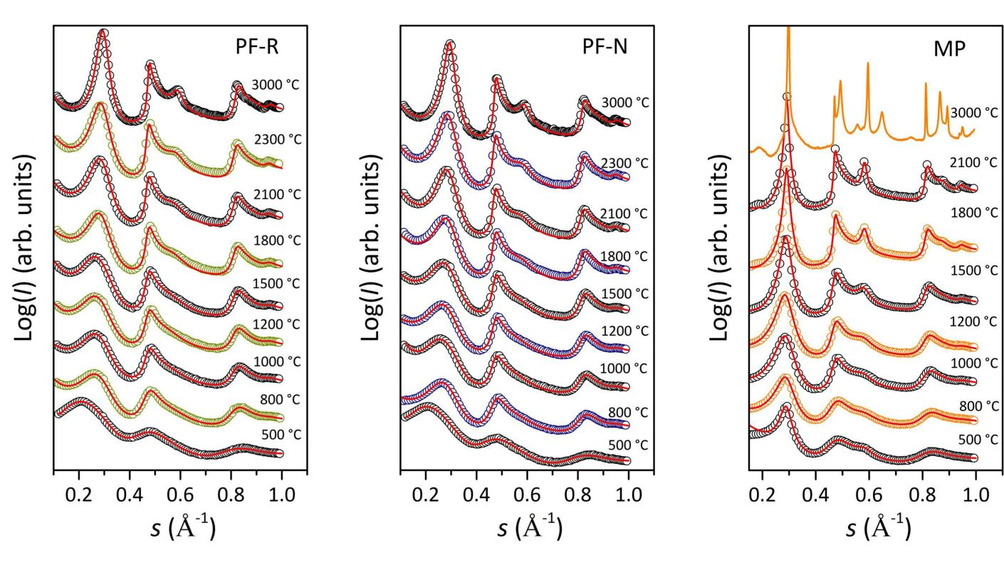
WAXS diffraction patterns: experimental data (circles), WAXS model curves (lines) as a function of the scattering vector  $s = 2 \sin(\theta) \cdot \lambda_{(Cu)}^{-1}$
