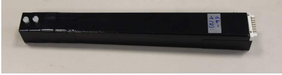
Figure 14: Wrapped crystal equipped with LAAPD and flange.
