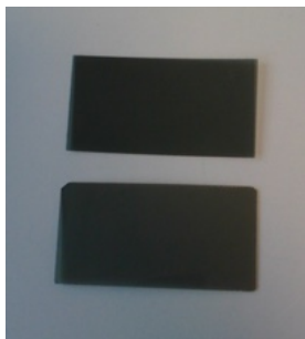
(a) Grey strip foil used as an optical filter.
