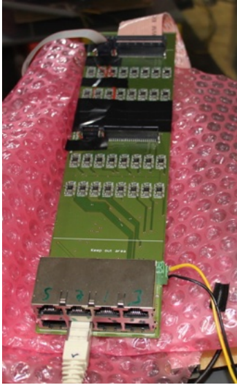
(a) Bufferboard with connected signal cables.
