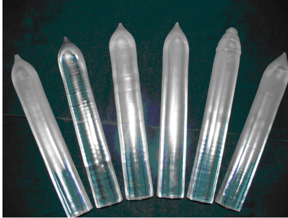
Figure 2.1: Lead tungstate ingots to produce modules in \overline{\text{PANDA}} geometry for the FEC [TDR].
