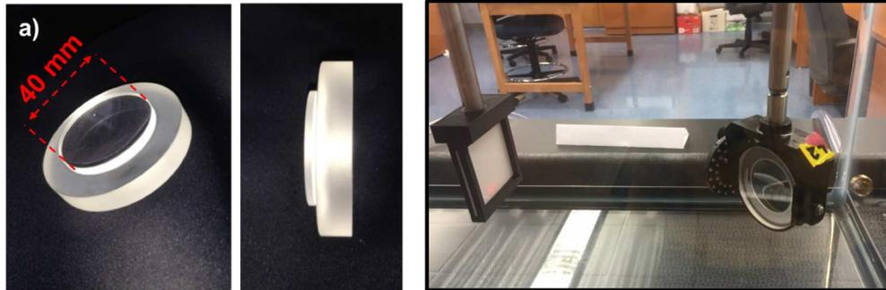
**Spherical 3-layer lens prototype**
