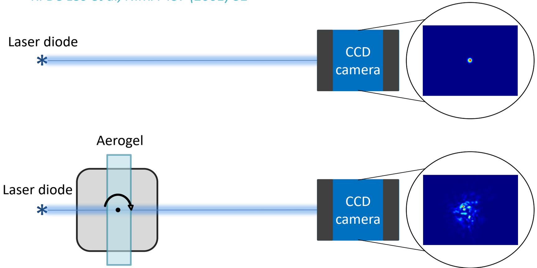
RMS scattering angle vs light path in aerogel
