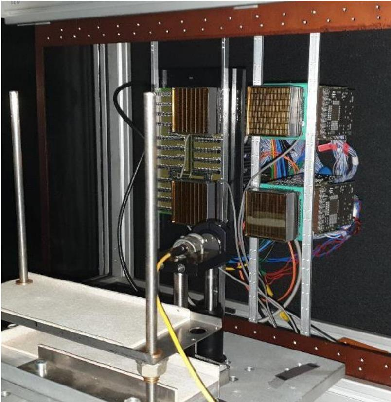
4 MaPMTs readout in half by PADIWA (128 ch) and DiRICH (128 ch)
