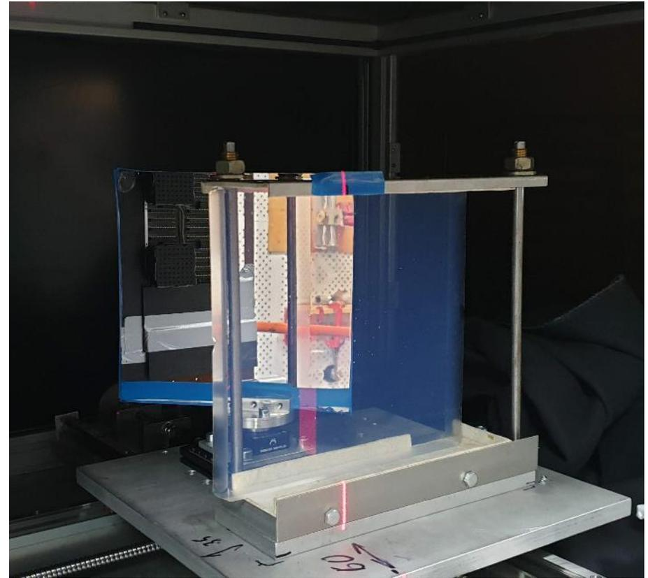
Aerogel sample with a flat mirror installed at 45° w.r.t. the PD and aerogel.
