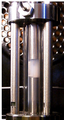
Figure: "Critical opalescence of ethane" by Dr. Sven Horstmann, used under CC BY-SA 3.0/cropped from original.
