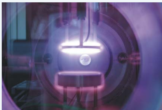
Capacitively coupled nitrogen/argon plasma (radio frequency) for the investigation of surface reactions under plasma conditions (S. Meiß/M. Rohnke, 2005)
