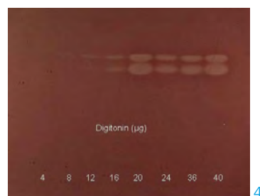
Hemolytic zones at white light: sample extracts (top) and digitonin concentration range (bottom, 4–40 \mu g/zone; outlier at 20 \mu g/zone; 2 zones, because a mixture of mainly digitonin and digaloinin).
