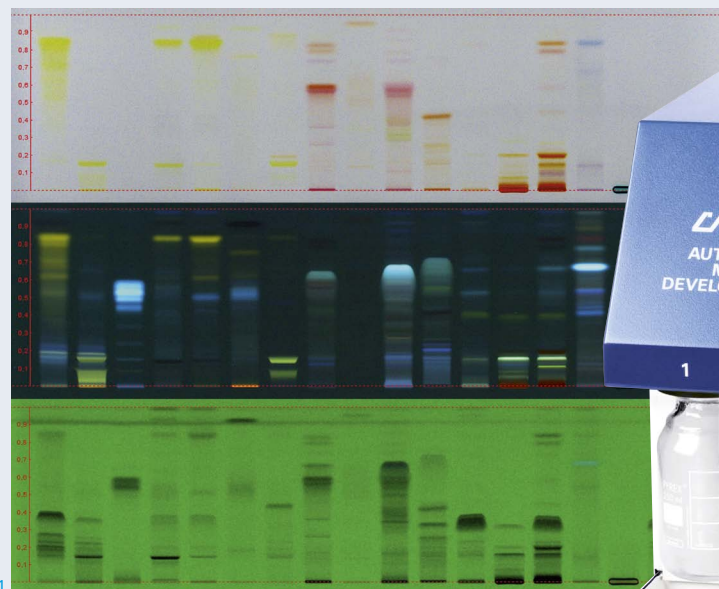
AMD 2 chromatogram of 18 organic pigments under white light, UV 366 nm and UV 254 nm; reprinted from [1], Copyright 2016 Elsevier; AMD 2-System (see application example on p. 4 in this CBS issue)
