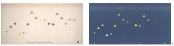
HPTLC plate after derivatization under visible light and under UV 366 nm for checking selectivity
