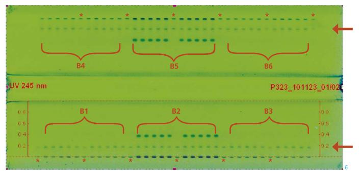
60 samples (6 batches, B1–B6) and 12 standards\* were applied onto one HPTLC plate; Coenzyme Q10 is seen at  $R_f \approx 0.20$ . In the Q10-batches on the center tracks vitamin B2 and vitamin E are also present ( $R_f \approx 0$  and 0.4); (\*NOTE: For better visualization in this figure the application volume was increased to 6  $\mu$ L).
