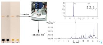
Extraction of a target zone with the TLC-MS Interface followed by LC-MS, total ion current chromatogram (TIC) of an apple extract spiked with a mixture of pesticides of various substance classes (A+) and mass spectrum of the peak with Rt=9 min (pirimicarb, m/z 239.1,  $[M+H]^+$ ).
