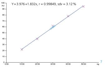
Calibration function for Coenzyme Q10 at UV 282 nm. Measurement of 10 samples and 5 standards using linear calibration (P323\_101011\_03).
