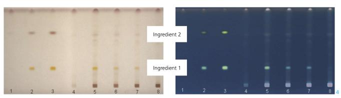
HPTLC plate after derivatization: Tracks 1–3 mixture of ingredients 1 & 2 for establishing the calibration function, track 4 blank, tracks 5–8 samples taken from 4 areas of a production vessel
