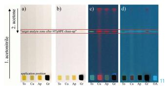
Separation of matrix and pesticides on TLC aluminum foils silica gel 60 NH<sub>2</sub>  $F_{254s}$  (tomatoes (To), cucumbers (Cu), apples (Ap) and red grapes (Gr); oleic acid (OA) was applied as a fatty acid example): before development under white light (a), after development under white light (b), UV 366 nm (c) and UV 366 nm after derivatization with primuline (d) (reprinted from [1] with permission).
