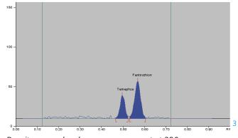
Densitogram, absorbance measurement at 290 nm
