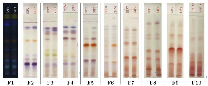
Optimized separation of polyphenolic fractions of Rh. officinale for coupling with TLC-MS interface
