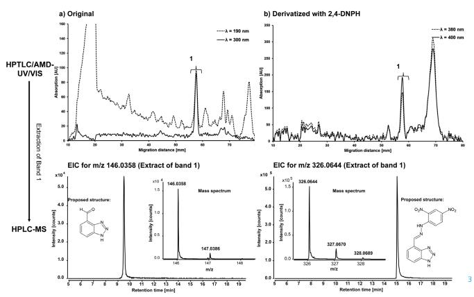
HPTLC/AMD-UV/VIS and HPTLC-HPLC-MS chromatograms and spectra: a) of underivatized and b) of derivatized oxidation byproduct M147 of 4-methyl-1H-benzotriazole
