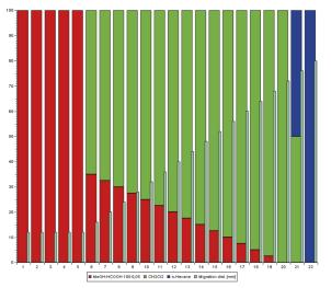
Diagram of the AMD gradient used for screening for oxidation by-products
