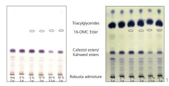
TLC images of ASE extracts for the detection of 16-OMC esters with vanillin sulphuric acid reagent (left) and phosphomolybdic acid reagent (right); track assignment: pure arabica coffee (Ara) and coffee blends with 2–50 % robusta coffee
