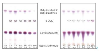
TLC images for the detection of 16-OMC with vanillin sulphuric acid reagent in ASE extracts analyzed following DIN 10779 (left) and direct saponification (right); track assignment: pure arabica coffee and coffee blends with 2–50% robusta coffee
