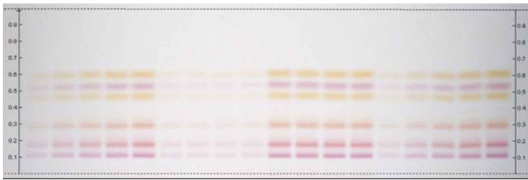
4 Chromatogram of Mix 1: The lowest and the highest concentrations were applied 5 times (center of the plate), the whole calibration range was applied in duplicate (on left and right side)
