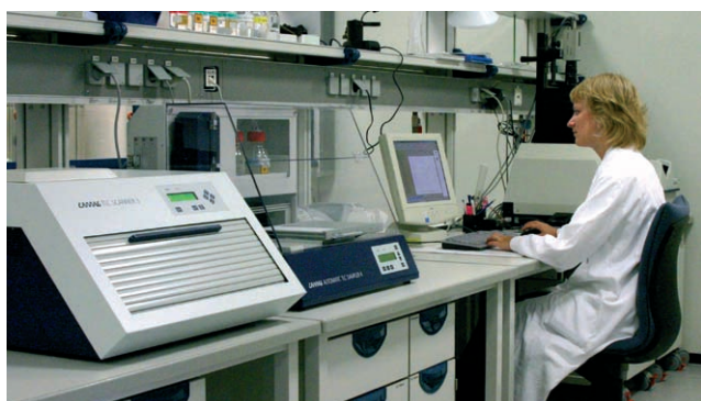
▲ Kerstin Armbrust is quantifying N,N-diethylethane-1,2-diamine in metoclopramide finished products at the HPTLC working place
