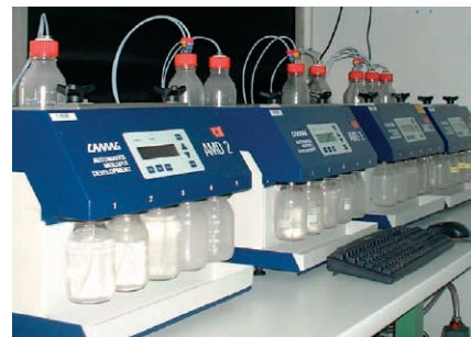
▲ For high throughput analysis of ceramides and lipids in cell culture samples four AMD2 systems are connected via a serial port to a personal computer.
