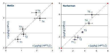
Fig. 2: HPLC/HPTLC correlations for the findings of MelQx (left) and norharmane (right) at five different cooking times T1 - T5: 3 min, 3 min 45 s, 4 min 30 s, 5 min 15 s and 6 min (mean value ± SD, n = 12, without outlier elimination)
