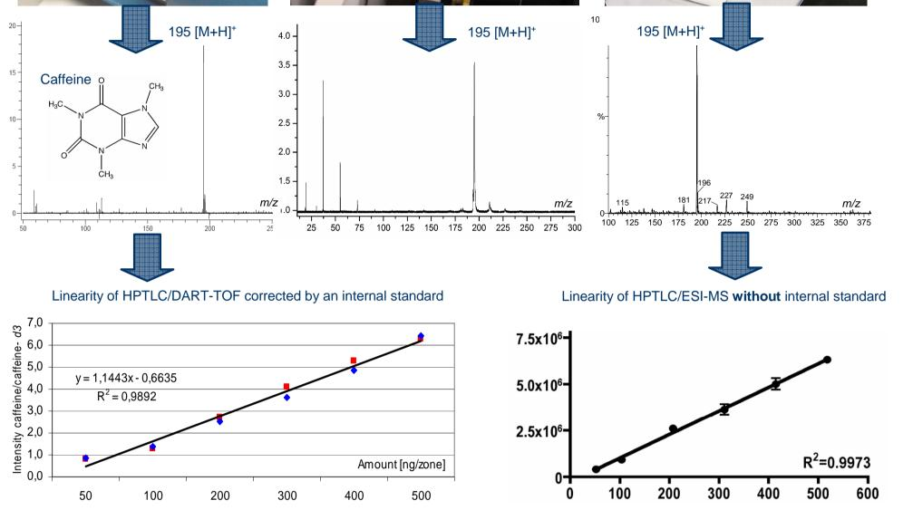
Fig. 1: Comparison of different ion sources, i. e. (A) DART, (B) APGD and (C) ESI, for HPTLC/MS coupling and their mass spectra (full scan) of caffeine @ m/z 195 [M+H]<sup>+</sup>. The analytical response (calibration ranged between 50 – 500 ng/zone) of HPTLC/DART-TOF had to be corrected by the internal standard caffeine-d3 @ m/z 198 [M+H]<sup>+</sup>, whereas HPTLC/ESI-MS showed a linear correlation without the use of an internal standard; experimental details see [3, 4].
