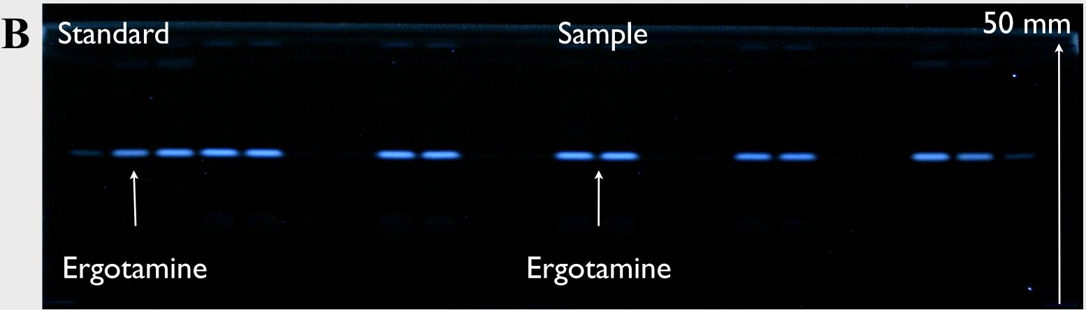
HPTLC plate silica gel 60 illuminated at UV 254 nm (A) and 366/>400 nm (B)
