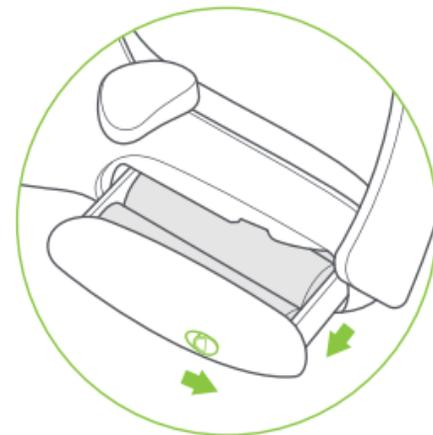
Slide the toggle according to arrow direction to open the battery case.
