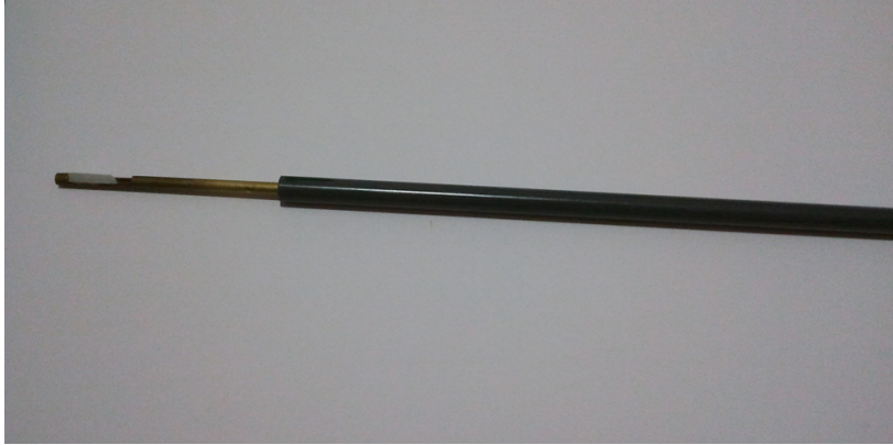
Figure 4.3: Closeup of one crystal sample already attached to the EPR holder.
