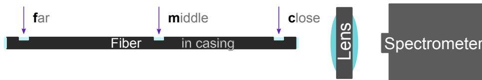
**Figure 3.3:** Schematic setup of the spectrum measurements of the DSB fibers.
