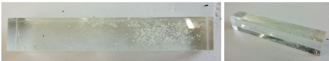
**Figure 3.19:** The block of DSB enriched with gadolinium with opaque, white spots inside.
