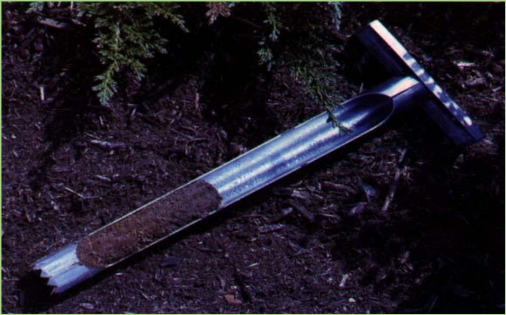
Soil corer with a diameter of 3 cm.
