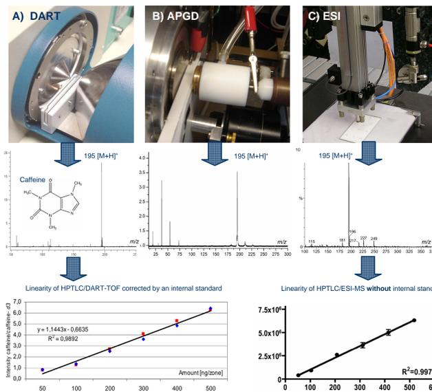
Fig. 1: Comparison of different ion sources, i. e. (A) DART, (B) APGD and (C) ESI, for HPTLC/MS coupling and their mass spectra (full scan) of caffeine @  $m/z$  195 [M+H]<sup>+</sup>. The analytical response (calibration ranged between 50 – 500 ng/zone) of HPTLC/DART-TOF had to be corrected by the internal standard caffeine-d3 @  $m/z$  198 [M+H]<sup>+</sup>, whereas HPTLC/ESI-MS showed a linear correlation without the use of an internal standard; experimental details see [3, 4].
