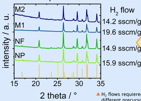
▲  $H_2$  flows required to reduce the different precursor morphologies.
