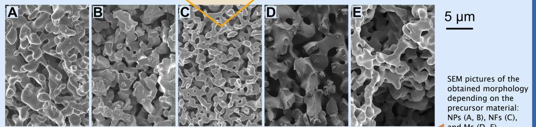
SEM pictures of the obtained morphology depending on the precursor material: NPs (A, B), NFs (C), and Ms (D, E).
