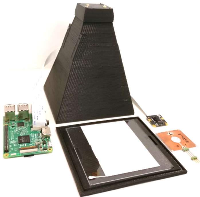
Visualization chamber: Raspberry Pi camera and UV-LED
